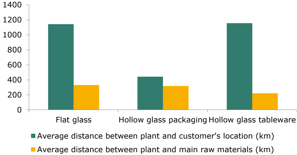
Figure 77. Average distance between plant and customer’s location and between plant and main materials (transport legislation)
